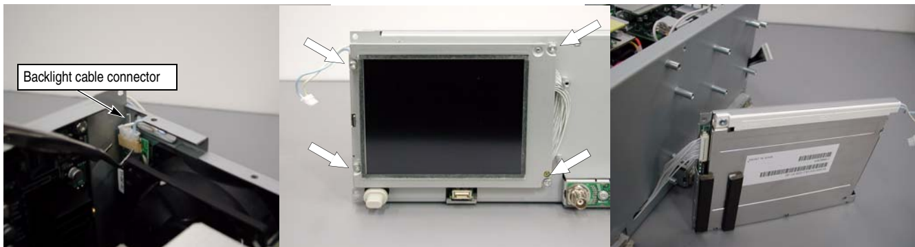
Figure 6-8: Display module removal
